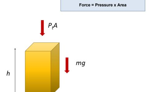
You may experience greater pressure as you go deeper into a swimming pool or in an ocean. What is the relation between pressure and depth? Let's consider one column of water with height h below the figure in a large swimming pool. The area (A) of the top face is the same as that of the bottom face. The pressure  $(P_t)$  on the top face creates a downward force or  $P_tA$ . The pressure  $(P_b)$  creates an upward force or  $P_bA$ . Also, the weight (mg) due to gravity points downward.
